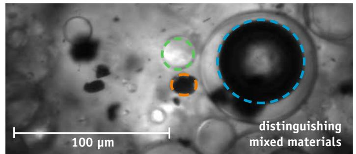
Real processes and materials vary in their properties and nature. Our intelligent software is able to distinguish between different materials and render separate size and characteristic distributions accordingly.
