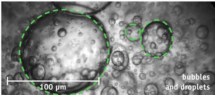
The properties of droplets in multiphase systems (e.g., water/oil) influence separation efficiency and mass transport. Knowing their size will enable you to minimize energy cost and waste.
