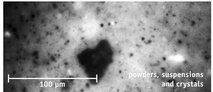
Undesired sizes of grain in processes can lead to costly product loss, damage in the machinery or filtration systems and lead to safety risks. Monitoring powders in real-time will give you enough time to react correspondingly.
