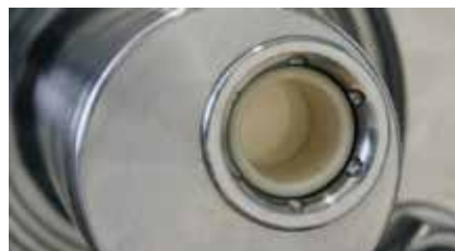
Probe retracted ( service position )
