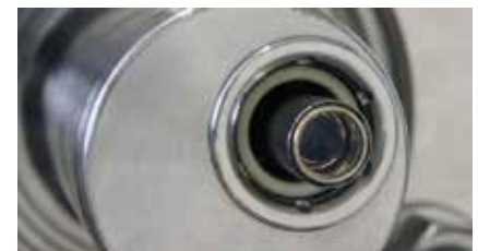
Probe extended ( measuring mode )
